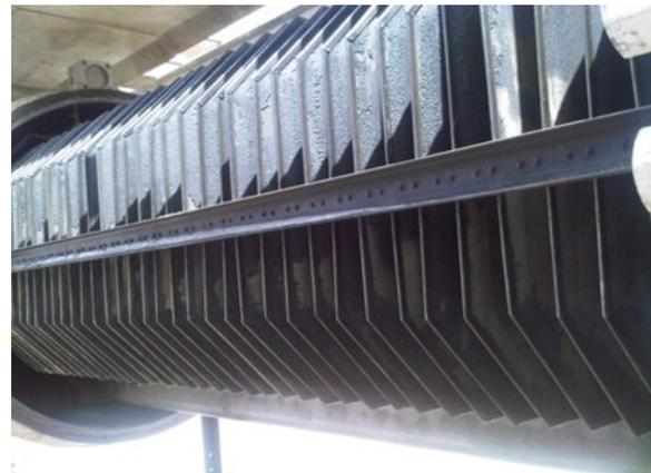
Picture 2: Plate & Frames partly "plugged" with pre-coat
